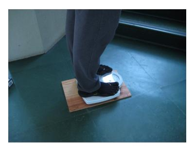
Part 2 - One side of the scale is propped on a stair or a similar rise so that when the student stands on the scale again, only the component of the student's weight perpendicular to the slanted scale is measured by the scale. The result is that the student appears to have "lost weight."
