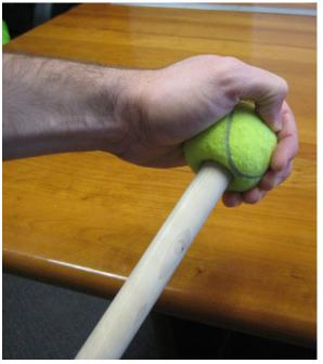
freedom a rod in a collar has is to slide and rotate along the axis of the rod. Lastly, the more flexible foam piece is used to demonstrate how a self aligning bearing is flexible enough to avoid exerting the reaction couples that a normal collar would. Note: the collar and self aligning bearing pieces are not pictured.
